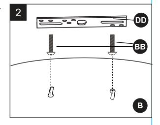
Attach crossbar (DD) to outlet box (not included) using short screws (AA).
